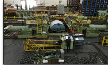
Unique capability to stretch and chem mill large structural components including skins
